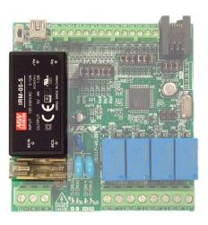
The DC version internally incorporates a voltage regulator:
